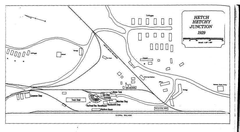
In 1925 headquarters for the construction work was moved from Groveland to Hetch Hetchy Junction, as the aqueduct line was stretched westward. The junction was in a narrow canyon, the only flat portion being that at the bottom of the map above. The upper legs of the railroad wye were
